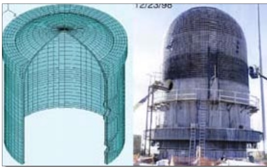
Specific features of modelling: allowing for reinforcement ropes in the form of thin sheets; calculation with account for concrete crusting
