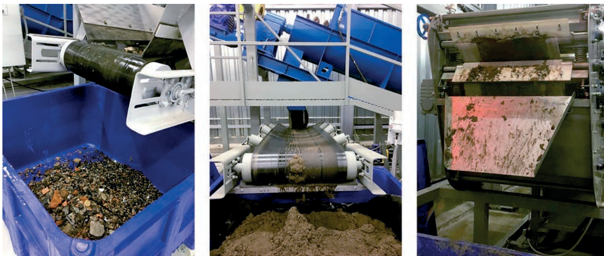
Figure 1. Unloading of processing products: a) from scrubber module with grain size of over 3 mm; b) from separator module with grain size of 0.15–3 mm; c) from filter-press module with grain size of less than 0.15 mm
