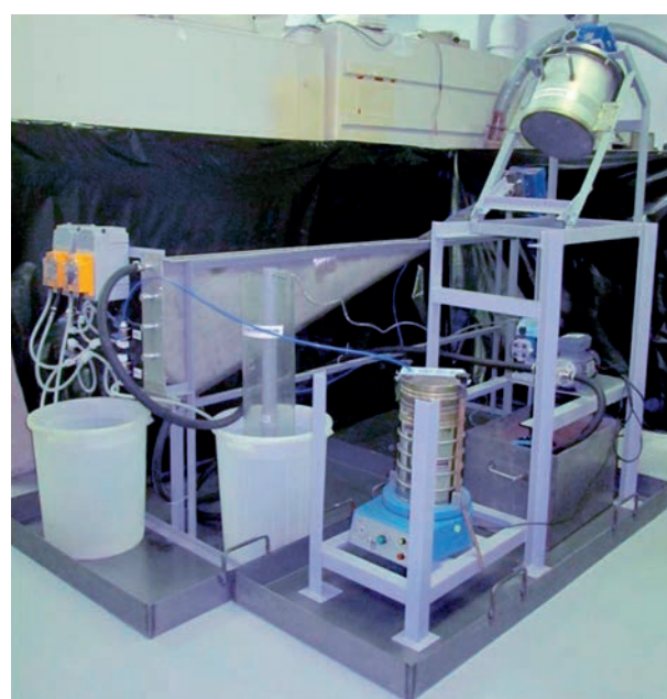
Figure 2. Laboratory test installation for RCS treatment via hydro-separation method
