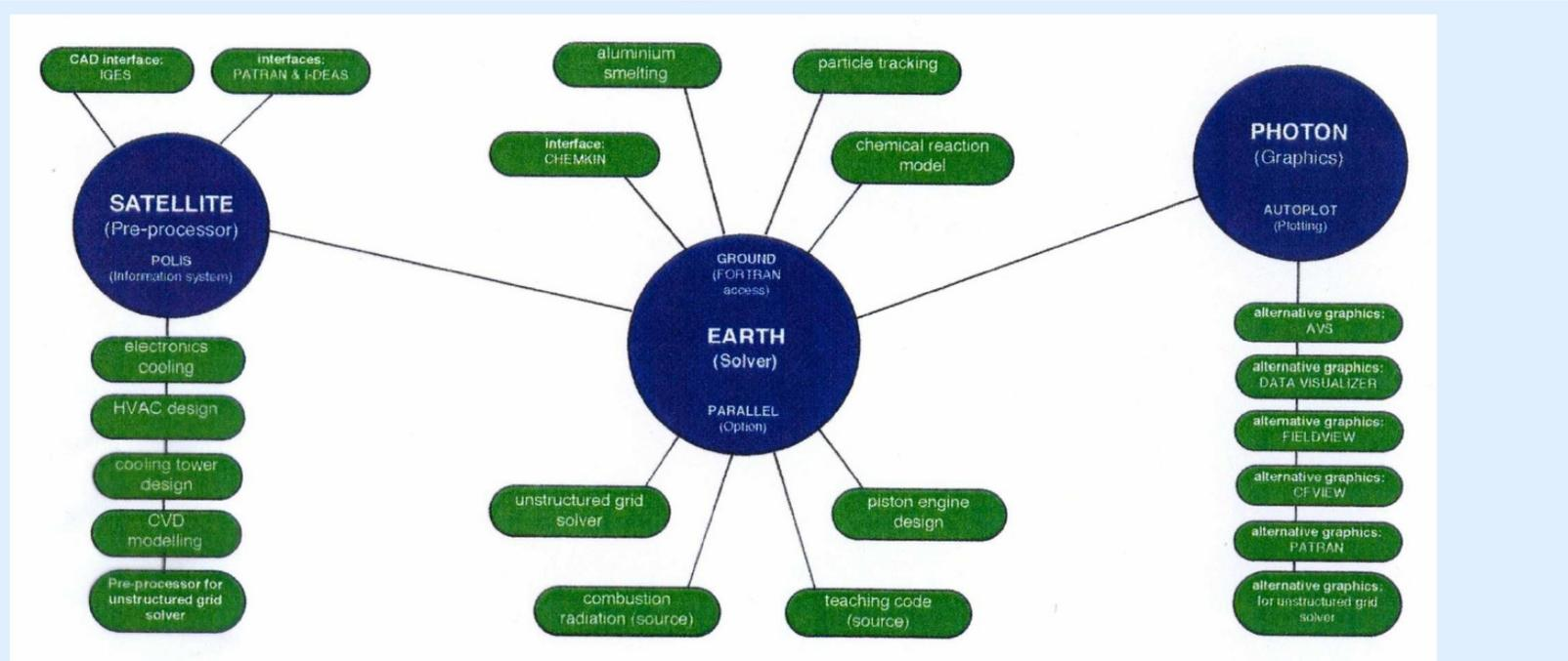
Modular design: **central solver** **pre-processor (mesh generator)** **post-processor (graphical display of results)** and modules to link in, as needed for the application.
